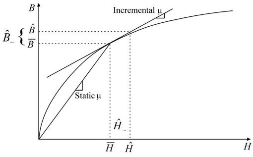
Permeability,  $\mu$ , is a material property by which  $\mathcal{L}$  varies with core size. Permeability is usually given in magnetics data as relative permeability,  $\mu_r$ . Then
